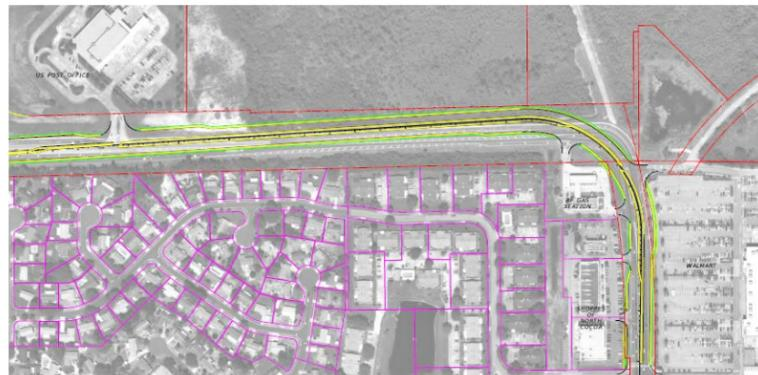
**35 MPH Curve:** This option introduces a curve that meets FDOT criteria for a 35 mph design speed. This curve will require additional right-of-way from the Walmart property and the existing BP gas station (not impacting the building or the station's functions).
