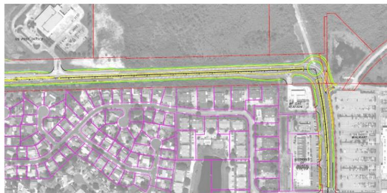
**Roundabout:** This option consists introduces a roundabout that meets FDOT criteria for a 20 mph design speed. Additional right-of-way will be needed from the vacant parcel north of Walmart.
